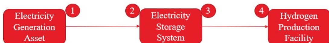
Figure 16: Schematic of the location of electricity meters for a Pathway using an Electricity Storage System.
